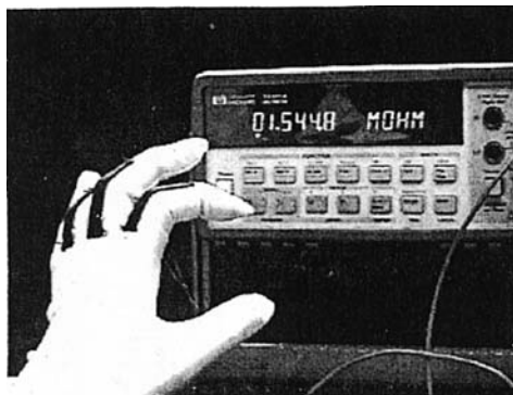
Figure 8 Prototype sensor glove with stretch fabric strain gauges attached to the metacarpo-phalangeal joints of each finger.
